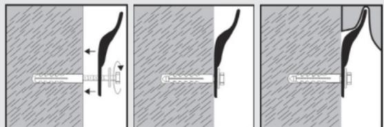
Use for corner basins or small hand rinse basins without large fixing holes in the basin back strap. The brackets, which are slotted for vertical adjustment, are designed to clamp on to the basin back strap and are supplied with screws and nylon plugs for solid walls. The screws can be used in to timber with a small pilot hole.
