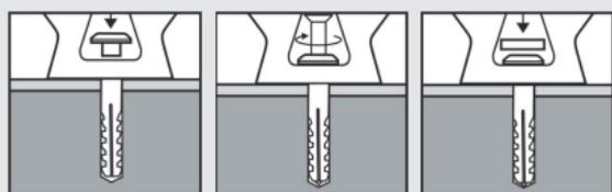
A conventional vertical fixing set for WC pans and bidets. The set includes a selection of nylon bushes and cover caps to accommodate different hole shapes and sizes. The brass screws can be used directly in to timber floors or with the nylon plugs supplied for concrete floors.
