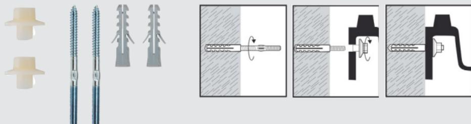
Use to fix small basins with large fixing holes to solid masonry walls. Can also be used to fix basins to partition walls where a timber frame has been built in to the cavity. For this application use the screw studs provided without the nylon wallplugs - a small pilot hole in the timber may ease installation.
