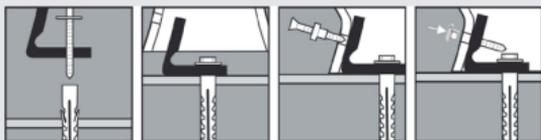
The fixing can be used to wall mount certain types of 'side fixed' ceramic trap covers or wash basin semi-pedestals.
