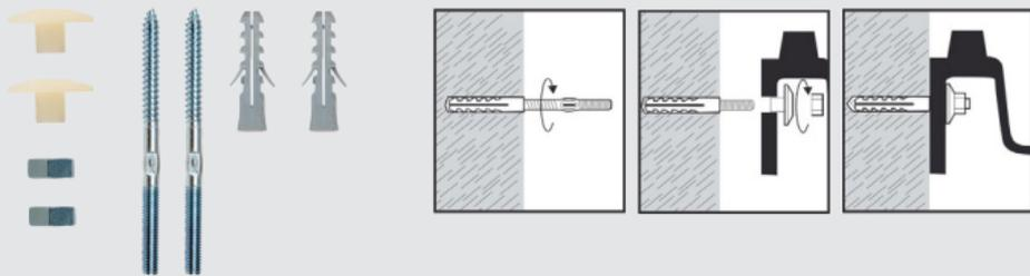
Use to secure wall mounted basins with large fixing holes to solid masonry walls. Can also be used to fix basins to partition walls where a timber frame has been built in to the cavity. For this application use the screw studs provided without the nylon wallplugs - a small pilot hole in the timber may ease installation.
